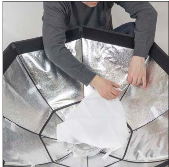
Now that the main structure of the softbox is complete, attach the inner-diffuser by using the Velcro tabs at located along the internal seam of the softbox backing material.
