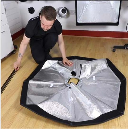
Lay the softbox backing material on the floor, and place the speedring in the center as shown in the image above.
