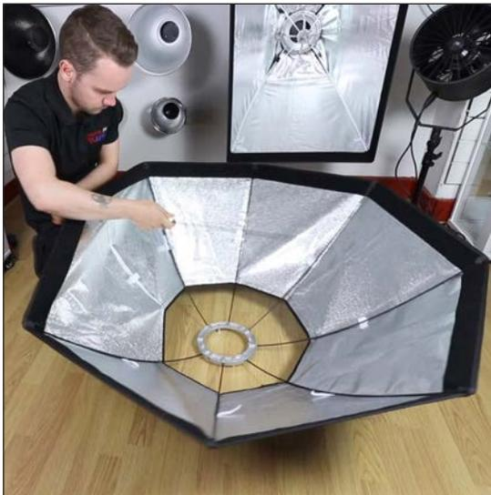
Now insert the remaining rods to complete the main structure of the softbox. P.S. Please be aware that the final rod will require a bit more force to insert than the rest due to added tension from the other three rods
