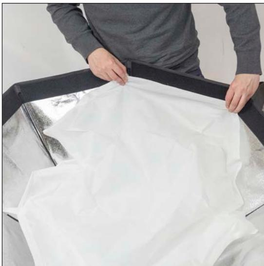
Once you have attached the inner diffuser, all that is left to do is attach the outer diffuser. To do this, simply attach it to the inner edge of the Velcro strip that goes around the internal perimeter of the softbox.
